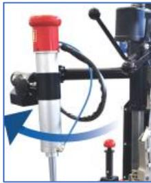
**BP1 Plus** pneumatic bead pressing arm. Lifts up automatically at the end of the mounting procedure, and moves back in rest position, with no need for the operator to change his working position (standard).
