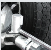
LL cylinder - for leverless demounting
